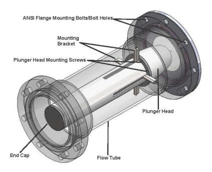
The End Cap (Figures 1 and 2) is at the inlet side of the valve. The downstream ANSI Flange (Figures 1 and 2) is toward the outlet side of the FluidDruid $^{TM}$  and, in some cases, a flange can be used to connect the valve to a fixture on the weir wall in the outlet control structure.
