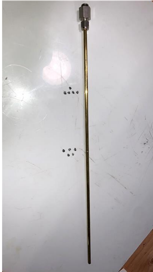
Figure 3-6: Insertion Rod for Plunger Displacement.
