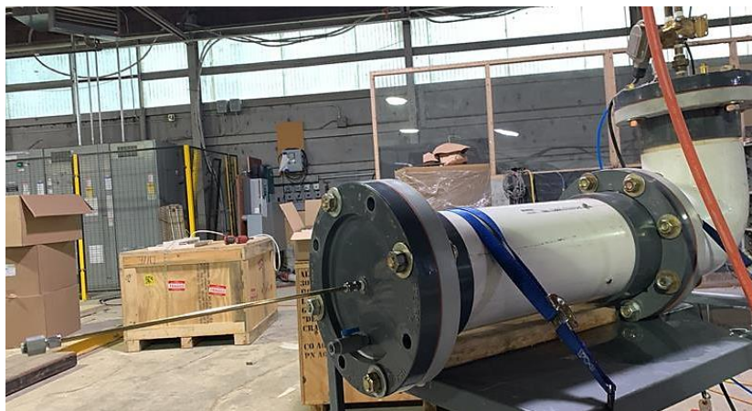
Figure 3-5: Cycle Test Chamber with SCH40 PVC and Insertion Rod
